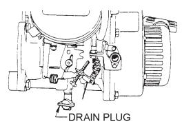
Figure 8. Drain Plug
